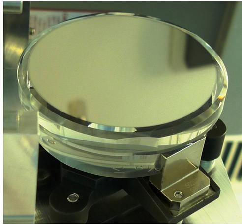
**Fig. 1:** Al/Mo/SiC coated primary mirror of High Resolution Imager of EUV telescope of Solar Orbiter.
